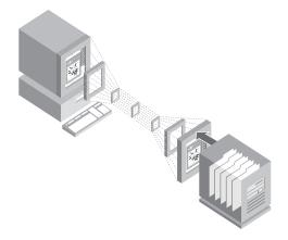
A highly efficient, remote presentation services protocol separates an application's logic from its user interface and allows only keystrokes, mouse clicks and screen updates to travel the network.
